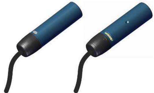
DOL 28R / iDOL 28R is a capacitive relay sensor for detection of feed, grain and solids in a feeding system. The sensor has relay output including switch function. The sensor has a white LED for illuminating the feed pan, a red LED indicating the status of the sensor and a green LED indicating it's powered on.
